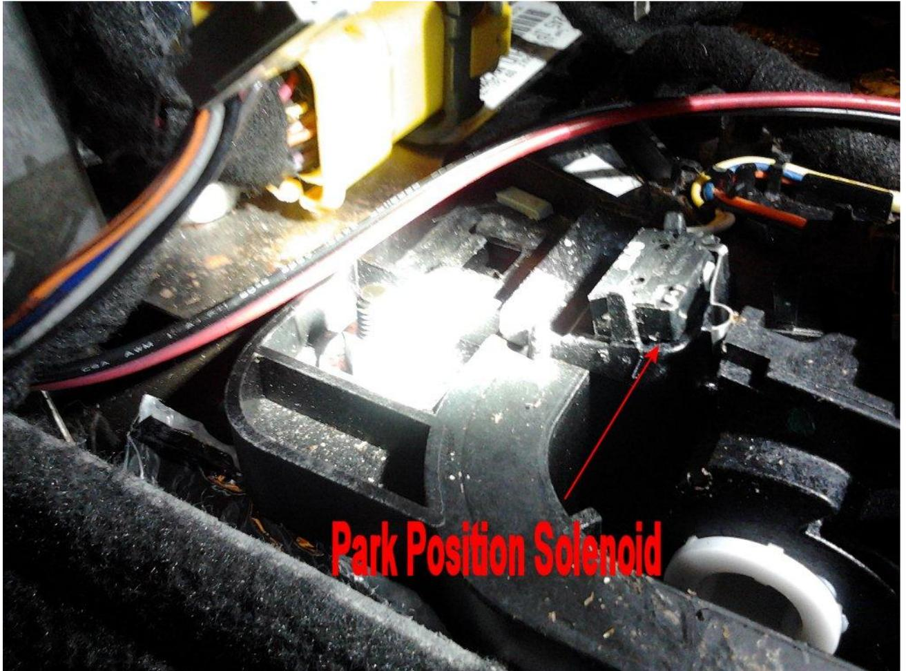
12) Assuming that your transmission is out of Park and stuck somewhere around Drive or Neutral. In order to release the Locking Pawl (tab), a small flat screwdriver can be inserted between the locking pawl and the catch, and pried up to get it released. Once this tab is released, then the shifter finger button can be pushed in, and easily moved into the Park position.
