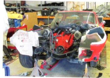
Then, while the repair work was in progress, some additional wreck related issues were found. The original Muncie transmission was locked up and the timing gear cover was damaged, among other things. Again, Mr. Baker reviewed the claim and promptly issued a second check.
